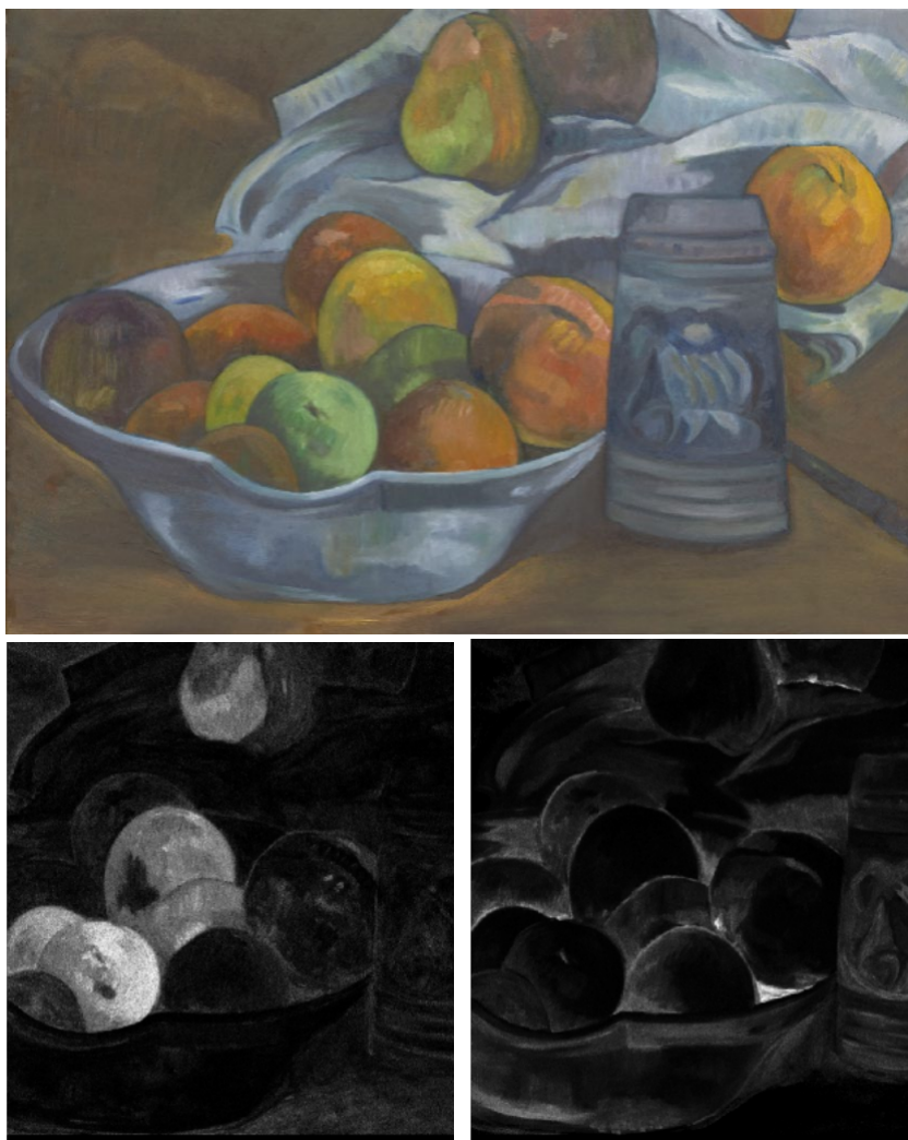
Figure 1: The RGB image at the top shows a sample painting made at the National Gallery, London. The two element maps at the bottom indicate with brighter colored pixels areas where different chemical elements are present in the painting. The image at the bottom left shows areas where barium is present, while the image at the bottom right shows areas where cobalt is present
